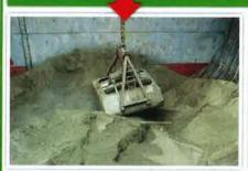
Copper concentrate exported to refinery for processing into metal
